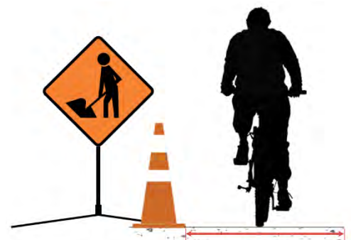
Figure 24 - Sign placement adjacent to vulnerable road user paths.
