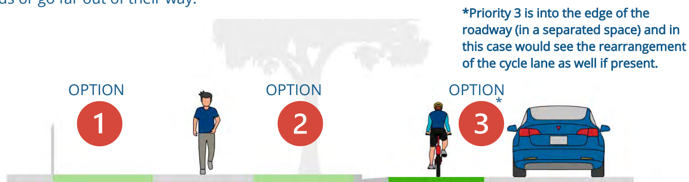
Figure 10 - Cross section of order of preference for pedestrian diversion options
