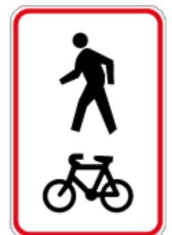
Figure 13 - R4-11 sign used to mark the start of a shared path.
